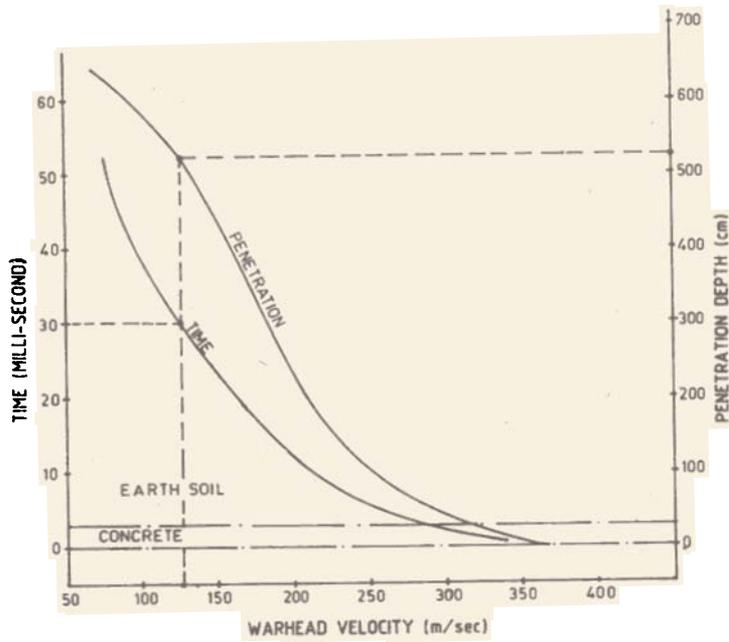
Figure 8. Space-time histories of warhead velocity during penetration process (Code : PEN).
