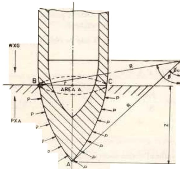
Figure 2. Part penetration of warhead into target medium.
