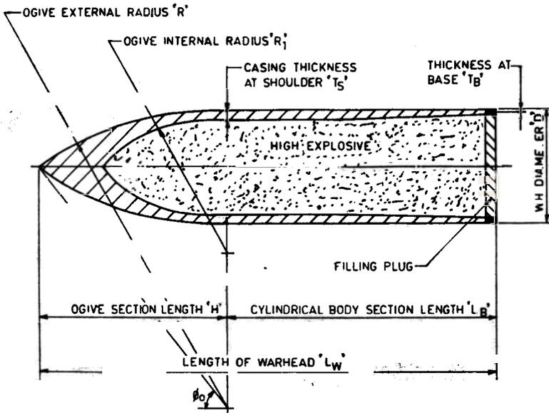
Figure 1. Elements of a typical earth penetrating warhead(EPW).
