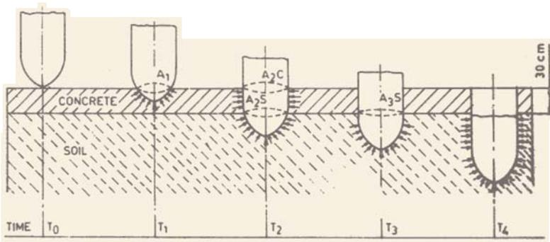
Figure 4. Representative sketch of the warhead penetration dynamics.
