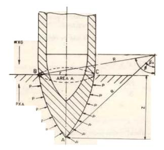
Figure 2. Part penetration of warhead into target medium.
