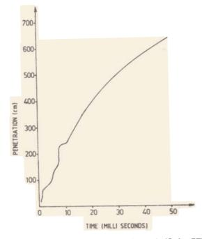
Figure 7. Warhead penetration on a time scale (Code : PEN).
