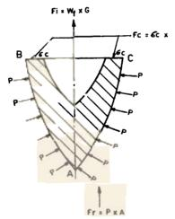
Figure 3. Free body diagram of penetrated part of the warhead.
