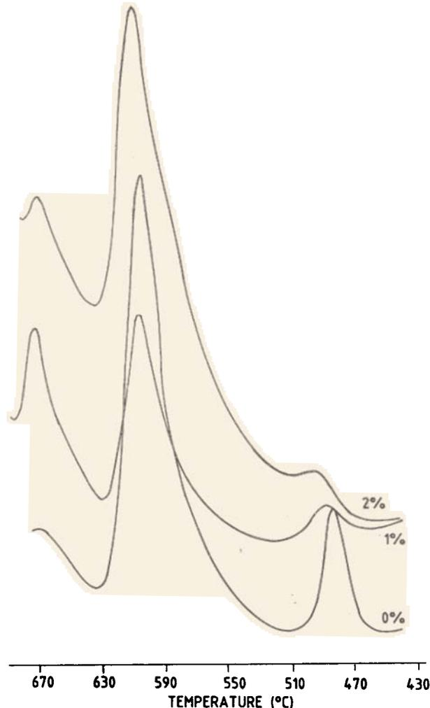
Figure 3. DSC of 60/40/15 at different binder contents.
