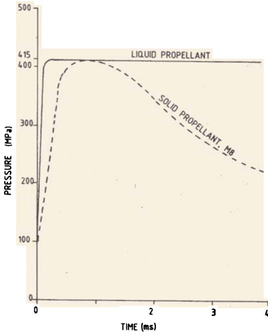
Figure 1. Pressure – time curves in a hypothetical 105 mm gun
