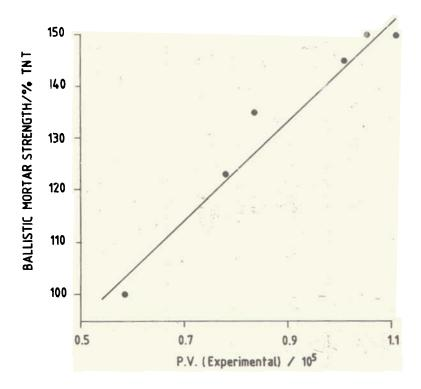
Figure 1 Regression plot of  $X_{pp}$  (4) vs. ballistic mortar strength data.
