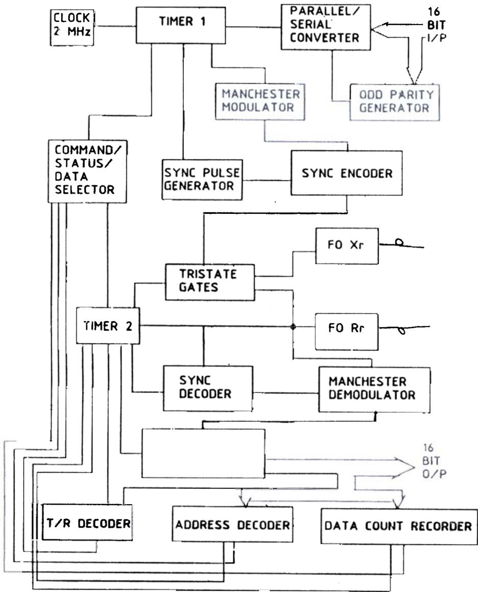
Figure 2. Block diagram of bus interface circuit
