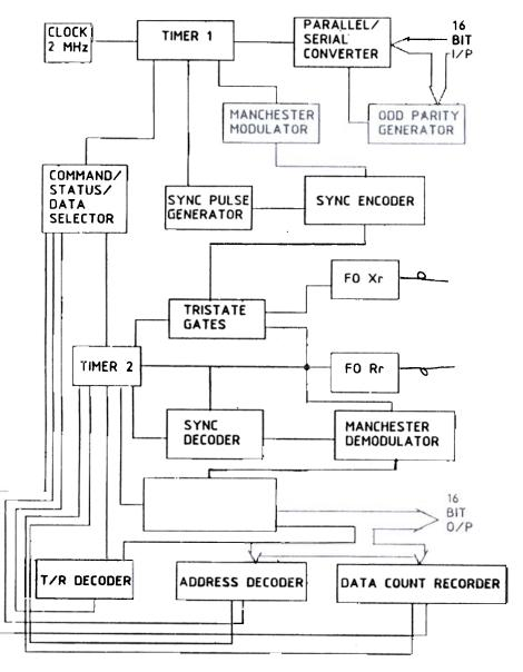
Figure 2. Block diagram of bus interface circuit
