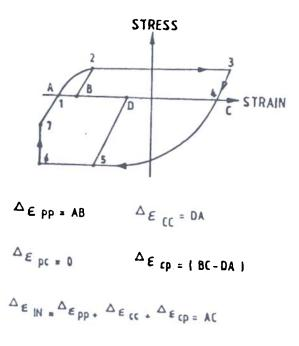
Figure 2. Partitioned of a complex hysteresis loop.
