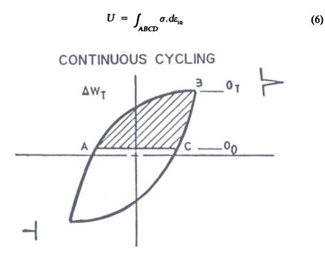
Figure 4. Schematic hysteritic loops defining net tensile hysteritic energy
