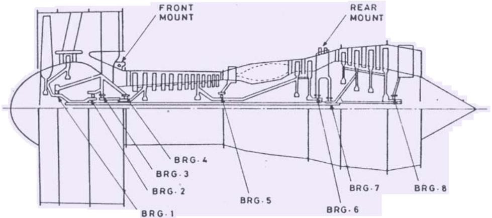
Figure 6. Twin-spool rotor-casing<sup>5</sup>
