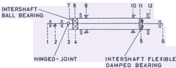
Figure 7(b). Idealised rotor with inter-spool damping<sup>10</sup>.
