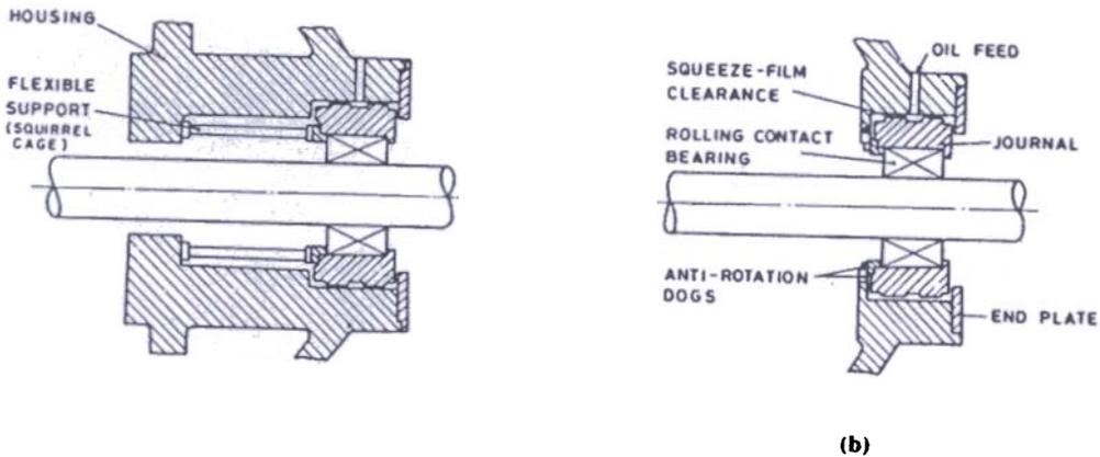
Figure 3. (a) Squeeze film damper with centralising spring and (b) Squeeze film damper without centralising spring.
