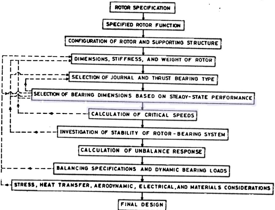
Figure 1. Logic diagram of design procedure<sup>1</sup>
