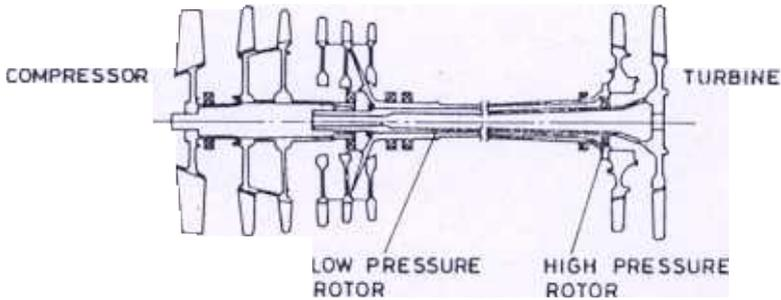
Figure 7(a). Rotor layout with inter-spool damping<sup>10</sup>.
