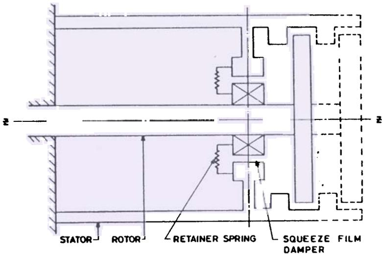
Figure 12. Overhung flexible rotor-casing model<sup>4</sup>.
