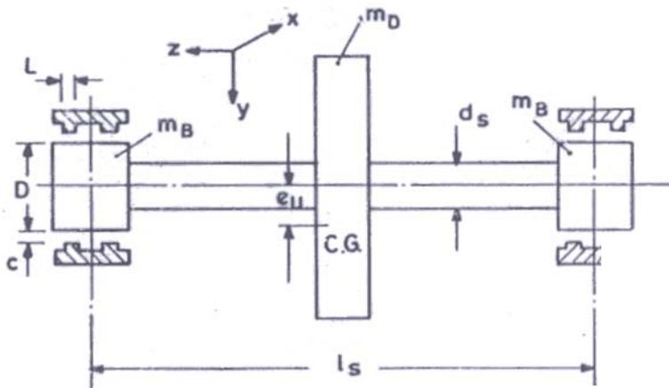
Figure 10. Rig/flexible rotor without centralising springs
