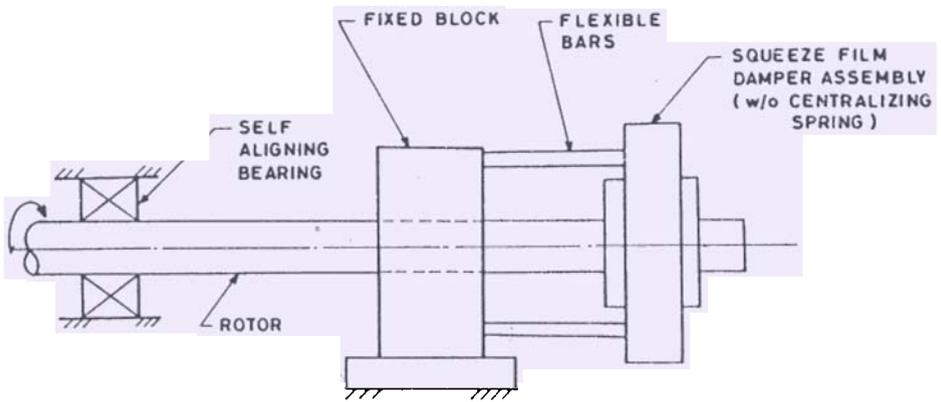
Figure 11 Unsymmetric rotor with squeeze film damping<sup>1</sup>
