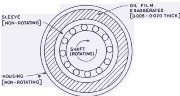
Figure 2. Elements of a squeeze film damper<sup>3</sup>.
