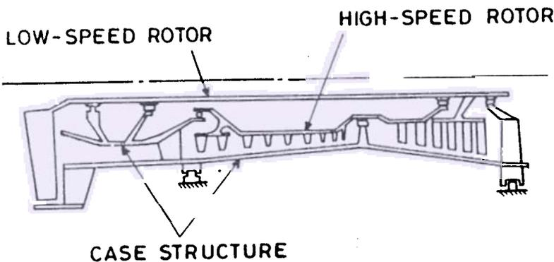
Figure 4(a). Twin-spool rotor layout<sup>7</sup>.
