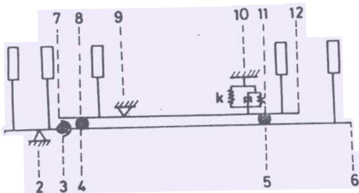
Figure 5. Twin-spool rotor layout<sup>6</sup>
