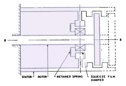
Figure 12. Overhung flexible rotor-casing model<sup>4</sup>.
