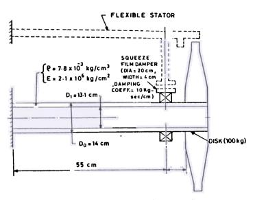
Figure 16. Overhung rotor for case study.
