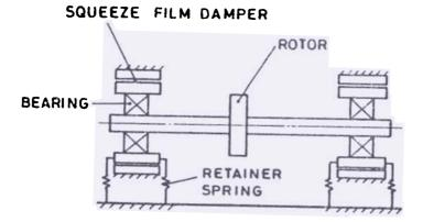
Figure 9. Rigid rotor with centralising springs
