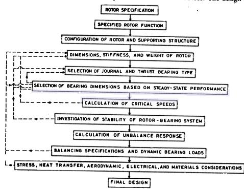
Figure 1. Logic diagram of design procedure<sup>1</sup>
