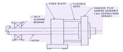
Figure 11 Unsymmetric rotor with squeeze film damping
