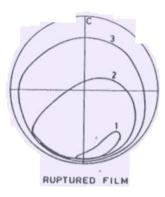
Figure 14. Typical steady-state orbits of a rotor without centralising spring.
