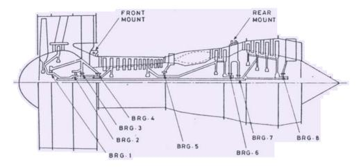
Figure 6. Twin-spool rotor-casing
