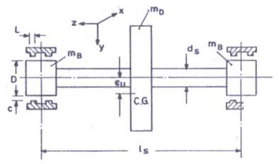
Figure 10. Rig/flexible rotor without centralising springs.
