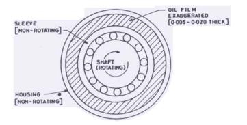
Figure 2. Elements of a squeeze film damper<sup>3</sup>.
