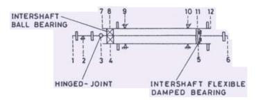
Figure 7(b). Idealised rotor with inter-spool damping<sup>10</sup>.
