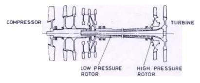
Figure 7(a). Rotor layout with inter-spool damping<sup>10</sup>.
