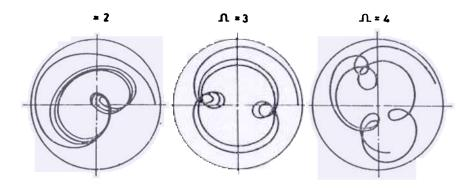
Figure 15. Typical subsynchronous orbits of a squeeze film damped rotor.
