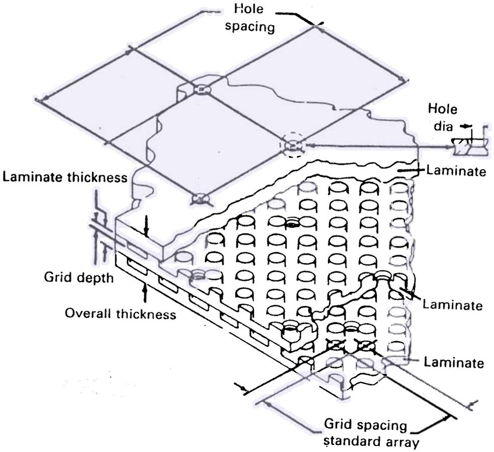
Figure 2. Typical geometric arrangement of laminated porous wall structure
