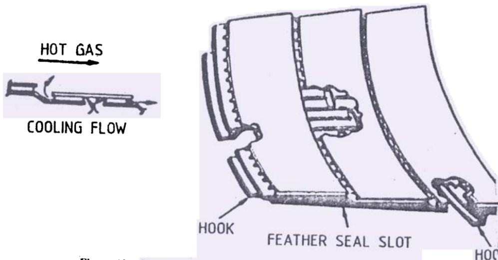
Figure 12. Segmented, counter-parallel FINWALL cooling scheme
