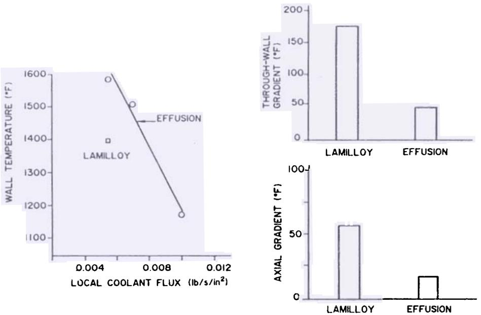
Figure 7. ATDE/GMA 500 reserve flow combustor test results with laminated porous wall and effusion cooling<sup>4</sup>.
