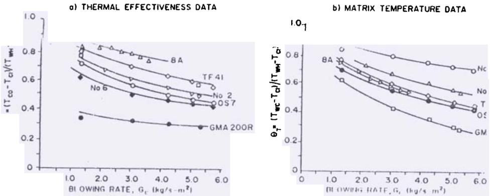
Figure 3. Thermal effectiveness and matrix temperature data for porous wall
