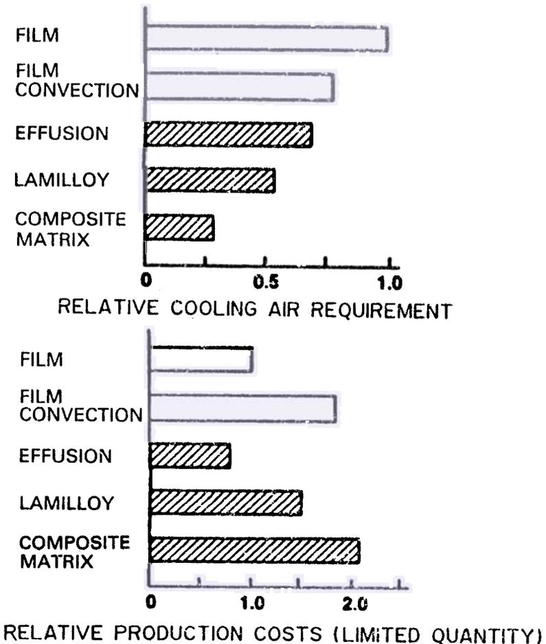
Figure 14. Cooling air requirements and production cost comparison of combustor liner cooling schemes<sup>4</sup>.
