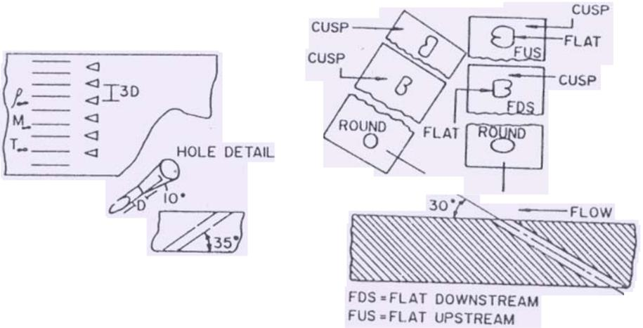
Figure 5. Shaped hole design configurations (a) Goldstein (Ref. 9), (b) Pappel (Ref. 10).
