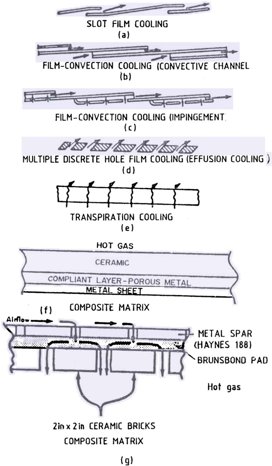
Figure 1 Combustor liner cooling schemes.
