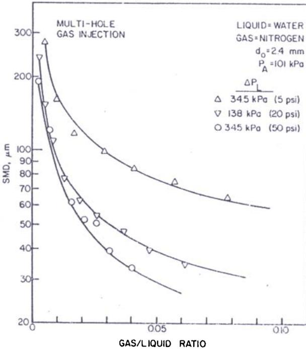
Figure 5. Influence of gas/liquid ratio and injection on SMD for  $d_0 = 2.4$  mm
