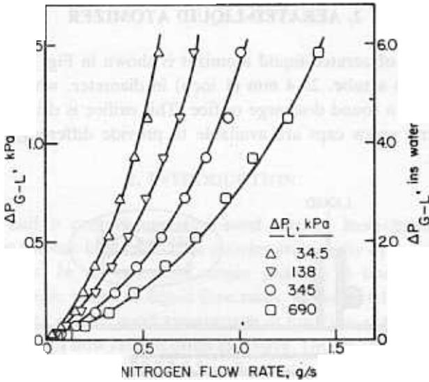
Figure 2. Pressure-differential between atomizing gas and liquid.
