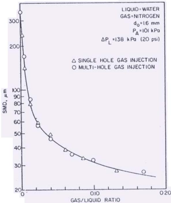
Figure 6. Effect of gas injector geometry on SMD for  $d_o = 1.6$  mm.
