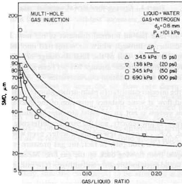
Figure 3. Influence of gas/liquid ratio and injection pressure on SMD for  $d_0 = 0.8 \text{ mm}$ .
