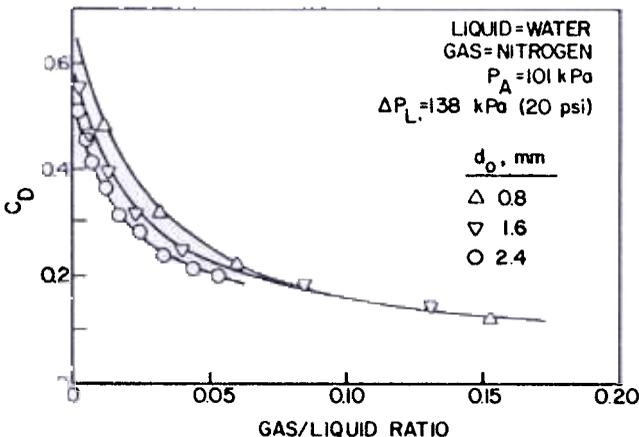
Figure 8. Effect of gas/liquid and injector orifice diameter on discharge coefficient.
