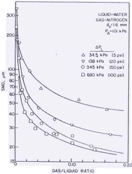
Figure 4. Influence of gas/liquid ratio and injection pressure on SMD for  $d_0 = 1.6$  mm
