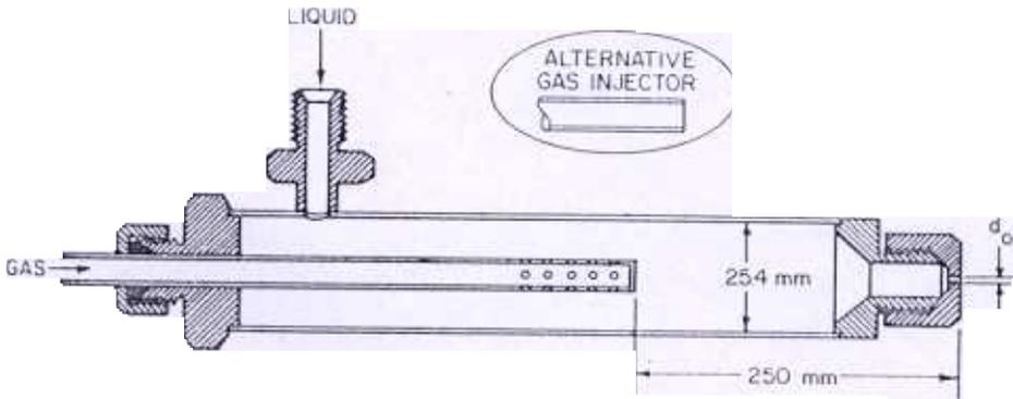
Figure 1. Cross sectional view of aerated atomizer.
