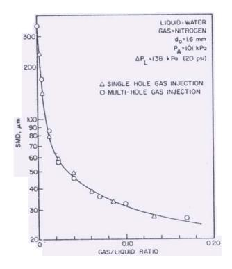
Figure 6. Effect of gas injector geometry on SMD for  $d_0 = 1.6$  mm.
