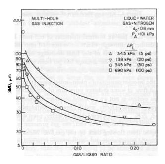
Figure 3. Influence of gas/liquid ratio and injection pressure on SMD for  $d_0 = 0.8$  mm.
