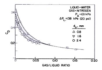
Figure 8. Effect of gas/liquid and injector orifice diameter on discharge coefficient.
