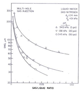
Figure 5. Influence of gas/liquid ratio and injection on SMD for  $d_0 = 2.4 \text{ mm}$
