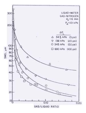
Figure 4. Influence of gas/liquid ratio and injection pressure on SMD for  $d_0 = 1.6 \text{ m}$
