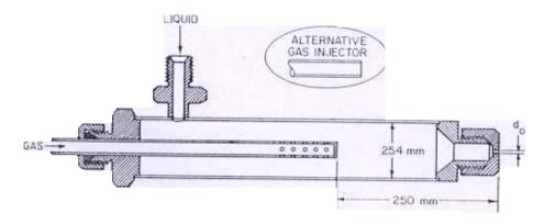
Figure 1. Cross sectional view of aerated atomic
