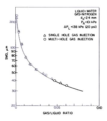
Figure 7. Effect of gas injector geometry on SMD for  $d_0 = 2.4$  mm.
