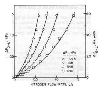
Figure 2. Pressure-differential between atomizing gas and liquid.
