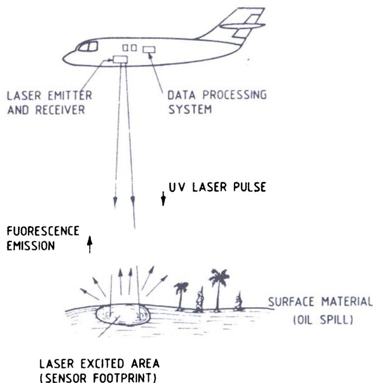
Figure Principle of airborne laser fluorosensing system.
