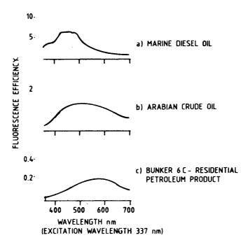
Figure 2. Fluorescence spectra of oils.
