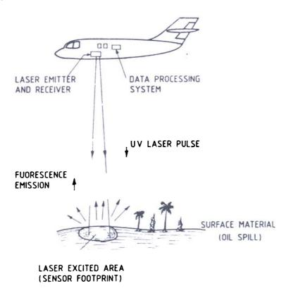
Figure Principle of airborne laser fluorosensing system.
