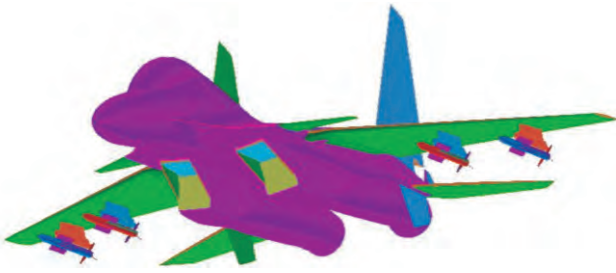
Figure 22. Aircraft with four missiles attached with the help of launcher and launch shoes.
