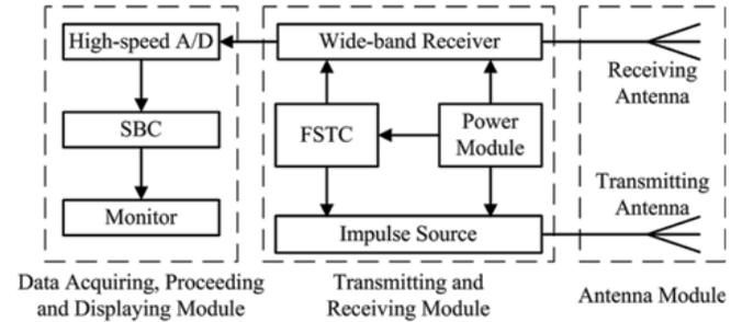
Figure 1. Block diagram of the impulse TWR.
