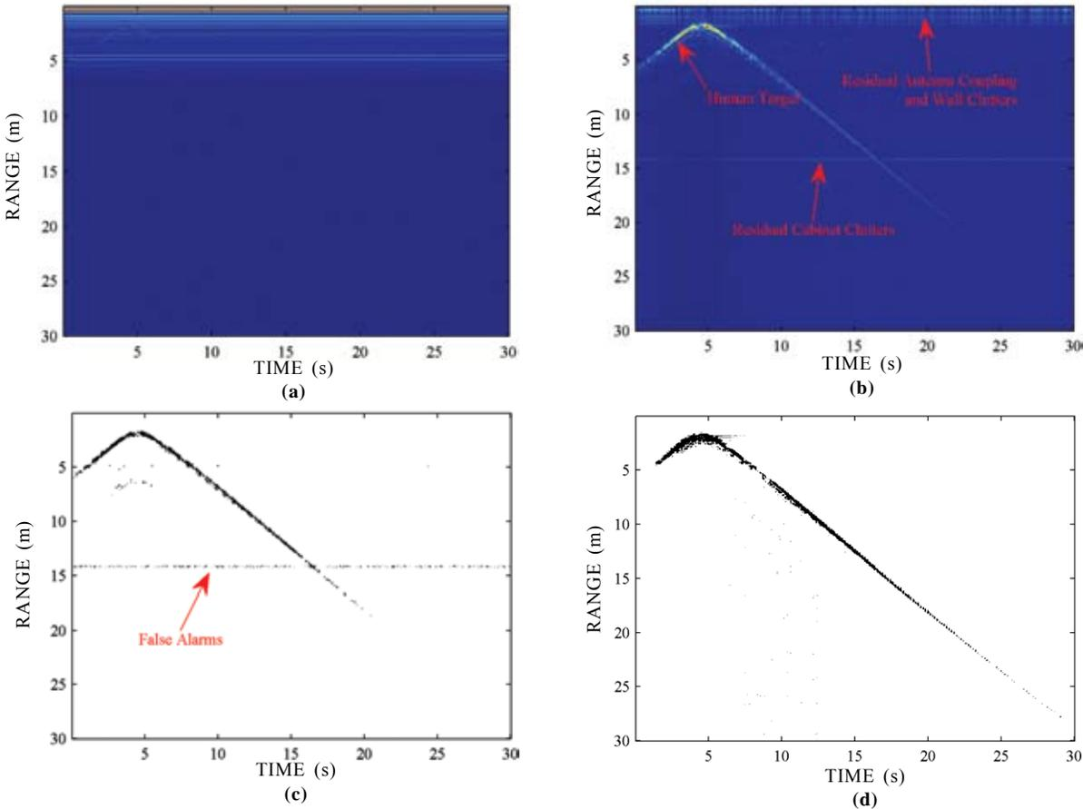
**Figure 5. Exponential results of one person moving behind wall. Range profiles of (a) raw data and (b) EABS processing result. Detection results using (c) the conventional OSCFAR method and (d) the proposed method.**
