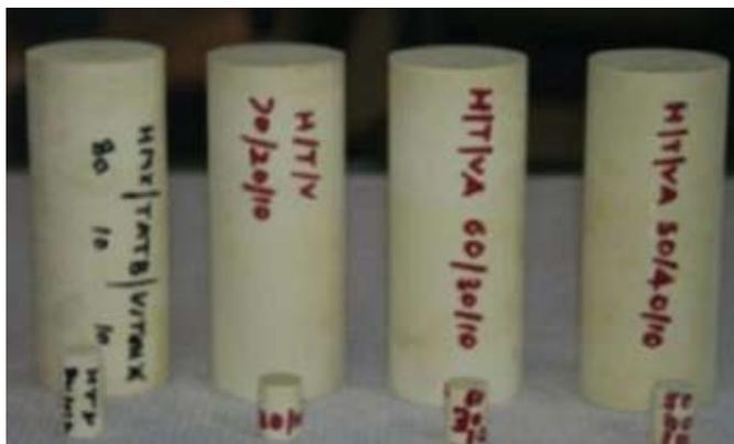
Figure 1. Photographs of some PBX compositions based on mixture of HMX and TATB.
