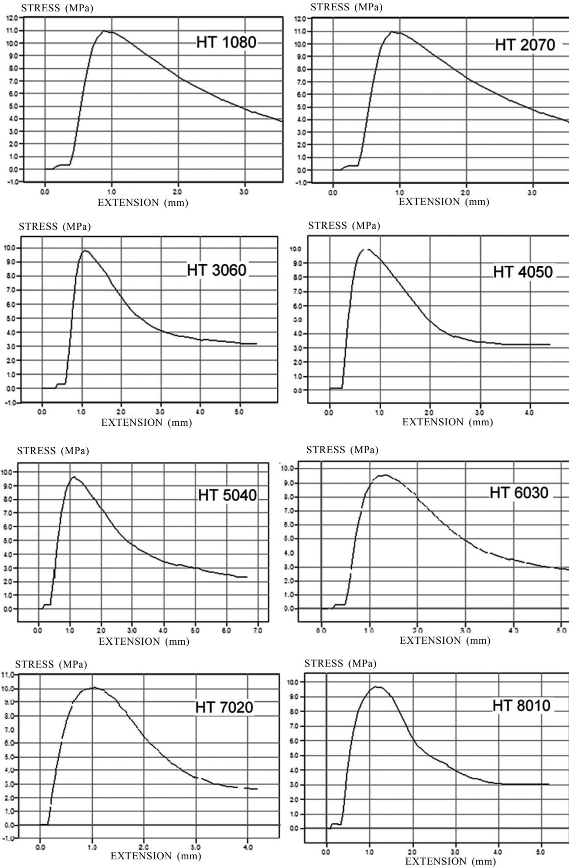
Figure 2. The compressive strength for PBX compositions based on mixture of HMX and TATB.
