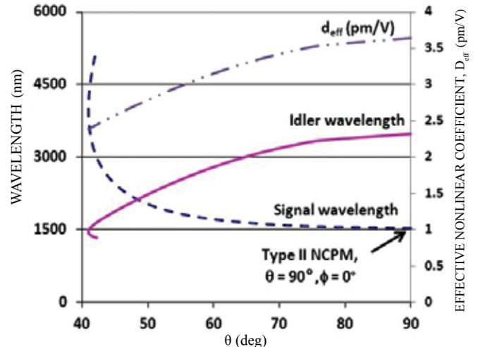
Figure 5. Calculated tuning curves in x-z plane for KTA-OPO pumped at 1064 nm.
