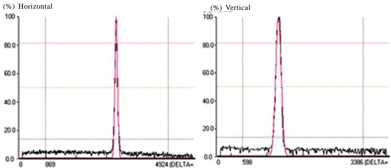
Figure 14. Far field spatial profile of eye safe laser.
