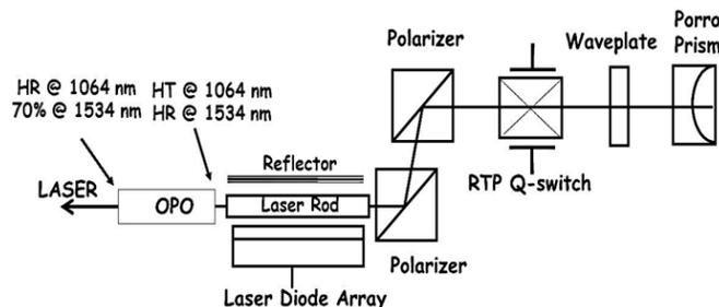
**Figure 1. Optical layout of laser resonator.**
