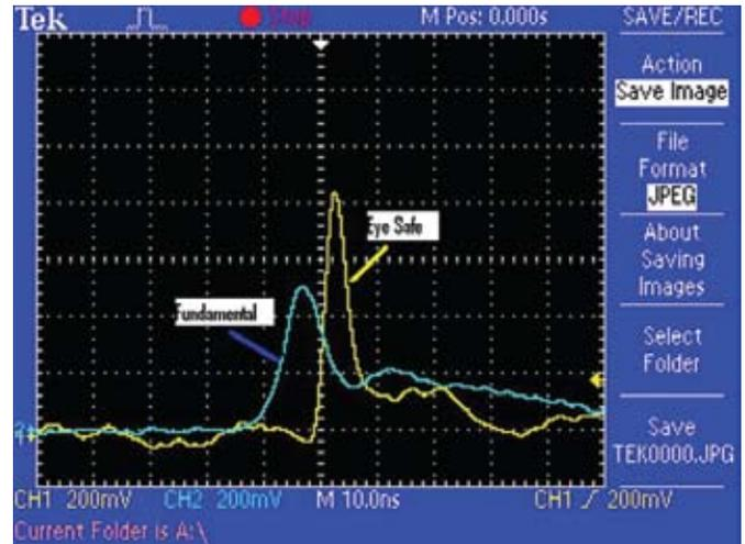
Figure 12. Pump and signal Q-switched laser pulses.
