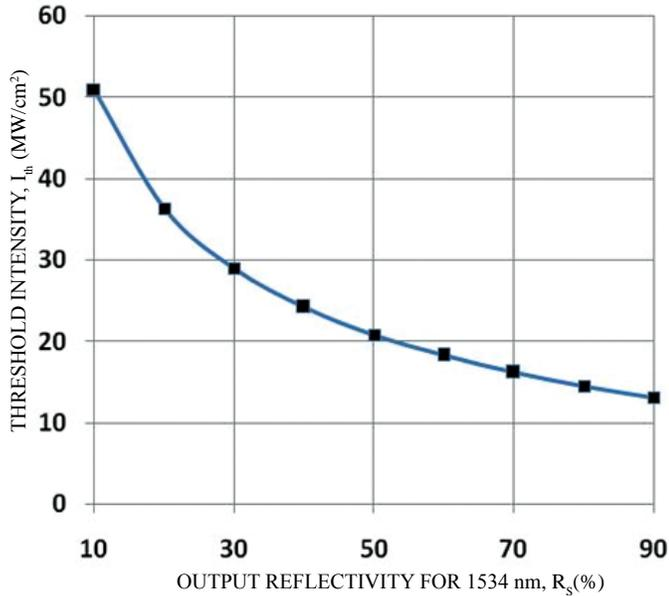
Figure 6. Calculated threshold intensity required for KTA-OPO eye-safe laser.
