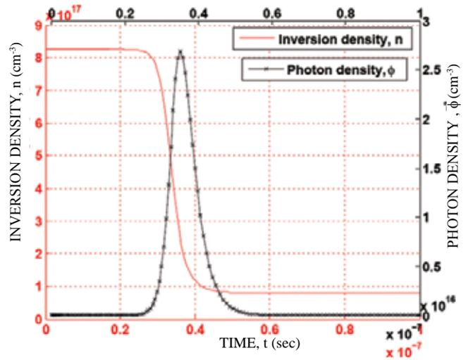
**Figure 2. Temporal variation of inversion density and photon density**
