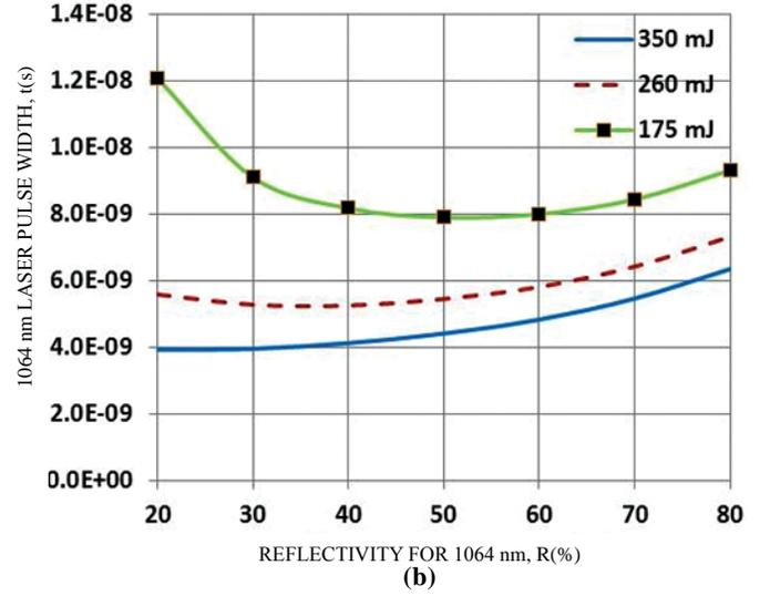
Figure 3. Variation of (a) output energy and (b) pulse width.
