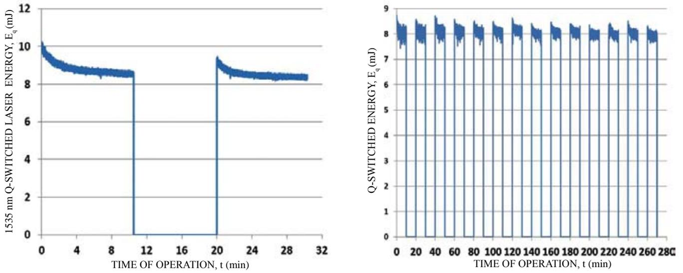
Figure 13. Signal laser at 20 Hz operation (a) 02 cycles, (b) 14 cycles.
