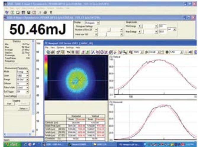
Figure 11. Free running spatial profile of 1064 nm output.
