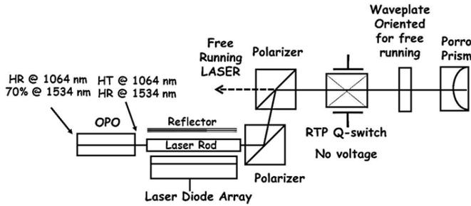
Figure 9. Free running resonator setup.
