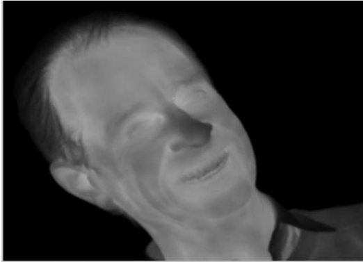
Figure 8. MWIR demonstration with 10 \mu\text{m} pixel pitch.
