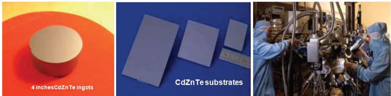
Figure 3. CZT ingots, substrates and MCT epitaxy layer process.
