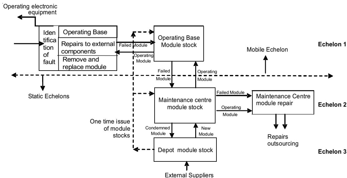
**Figure 5. Three-echelons model with one repair centre.**
