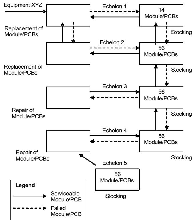
**Figure 3. Defective module/PCB flow diagram of equipment xyz.**
