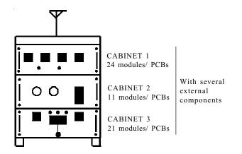
Figure 2. A telecommunication equipment xyz having three cabinets.
