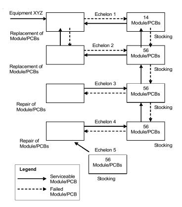
Figure 3. Defective module/PCB flow diagram of equipment xyz.
