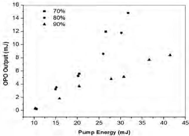
Figure 4. Energy scaling of OPO at different reflectivity for degenerate case.
