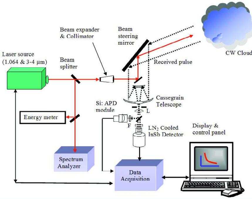
Figure 2. Schematic diagram of differential absorption LIDAR (DIAL) system.
