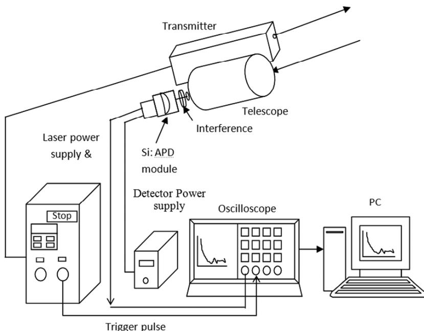
**Figure 1. Block diagram of backscattering LIDAR system developed at LASTEC, Delhi.**
