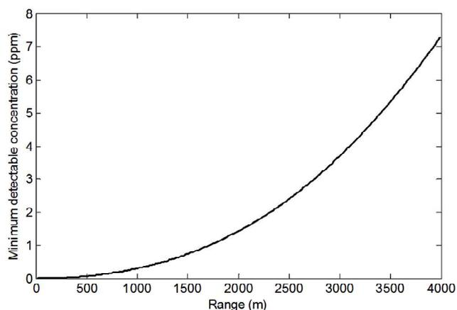
**Figure 3. Minimum detectable concentration versus range computed for tabun agent using DIAL technique.**
