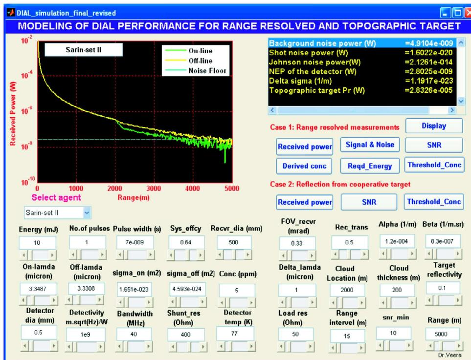
Panel 2. Graphical user display panel developed for DIAL system modelling.
