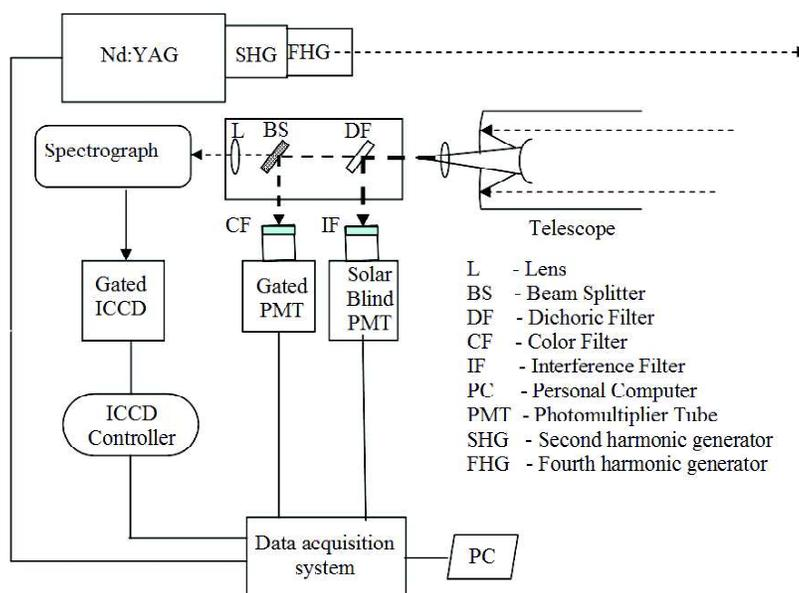
**Figure 4. Block diagram of the UV LIF LIDAR system.**
