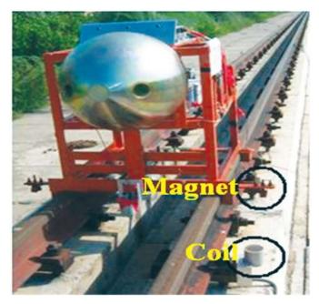
Figure 1. Deployment of sensor along the track.
