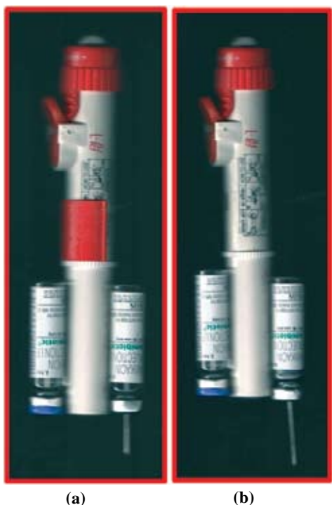
Figure 1. Autoinjectors with drug cartridges (a) Autoinjector with the restrictor for the partial delivery of the drug with partially ejected needle. (b) Autoinjector with fully ejected needle.
