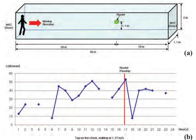
Figure 3. Test environment and initial experiment result: (a) test environment of location tracking, (b) an example of walking speed ZigBee tag experiment results without mediation.
