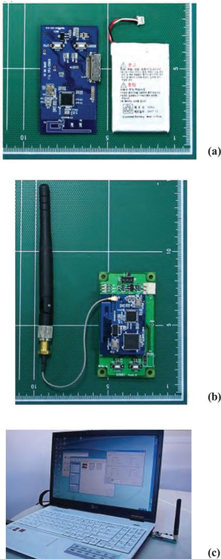
Figure 2. (a) ZigBee tag, (b) router, and (c) personal computer with gateway.
