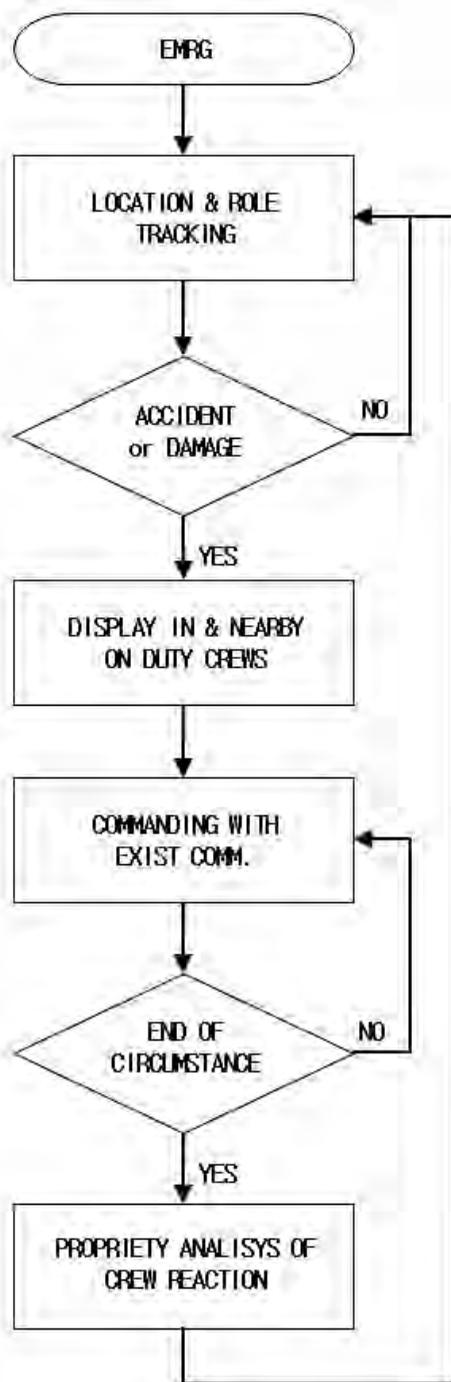
**Figure 1. Flow chart of a damage control concept using crew member location tracking.**
