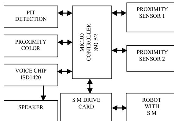
Figure 1. Integration of a microcontroller.
