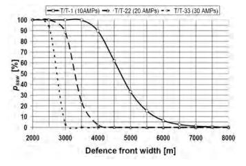
Figure 5. Successful swarming probability as function of defence front width.
