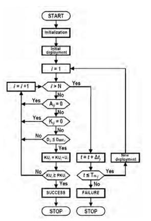
Figure 2. Basic swarming simulation algorithm (monotarget/ threat).
