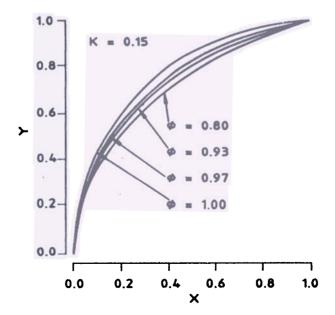
Figure 2. Minimum drag shapes are drawn for various values of shape parameter and known values of K = 0.15.
