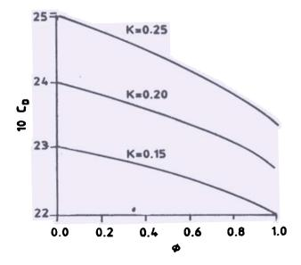
Figure 4. Relationship between  $C_D$  and shape parameter  $\bigoplus$  for K = 0.15, 0.2 and 0.25.
