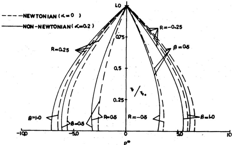
Figure 8. Pressure coefficient on either disc versus  $\xi/\xi_0$  for  $R = -0.5, -0.25, 0.25, 0.5$  and  $\beta = 0.5, 1.0$ .
