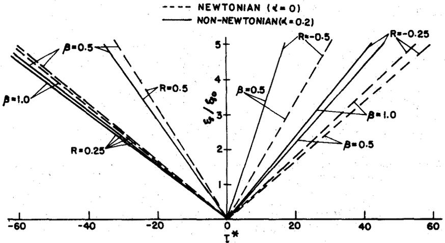
Figure 9. Coefficient of skin friction at the upper disc versus  $\xi/\xi_0$  for  $R = -0.5, -0.25, 0.25, 0.5$  and  $\beta = 0.5, 1.0$ .
