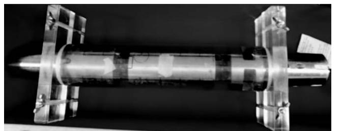
Figure 4. (a) Schematic, and (b) actual load balance of type-D.
