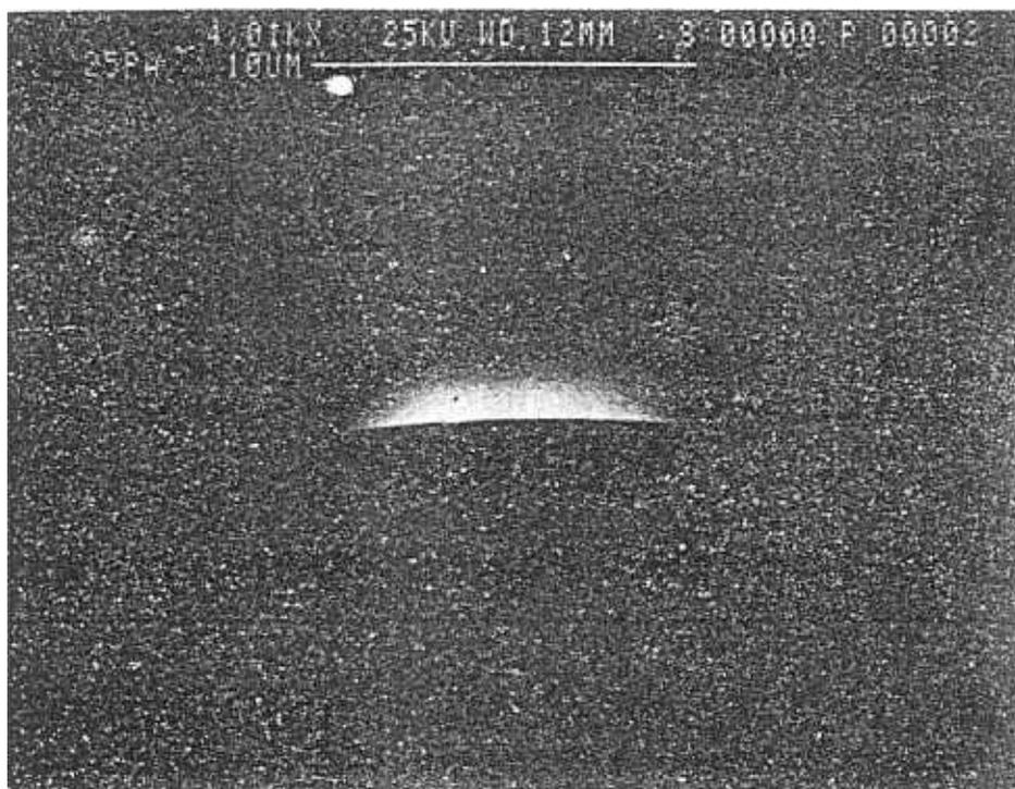
Figure 10. A typical oval defect related to the Ga cell in MBE-GaAs.
