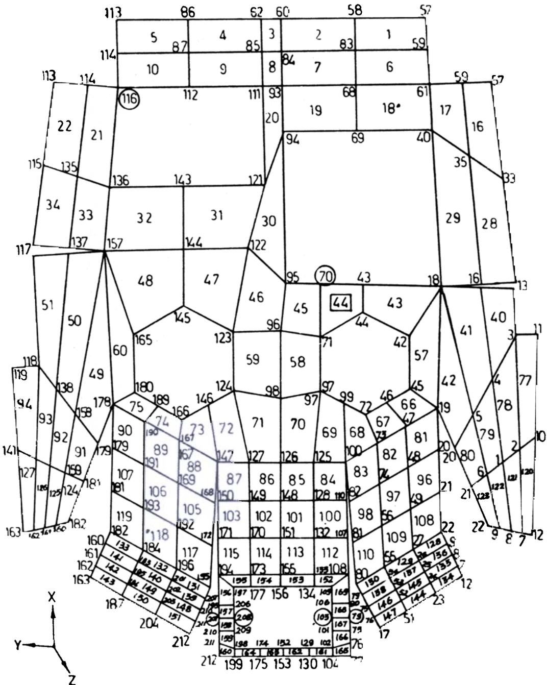
Figure 2. Turret discretization (top and four side plates).
