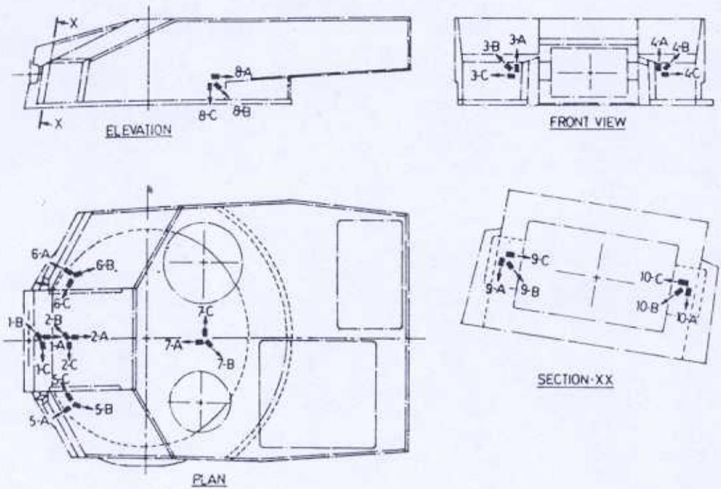
Figure 5. Strain gauge locations on turret model.
