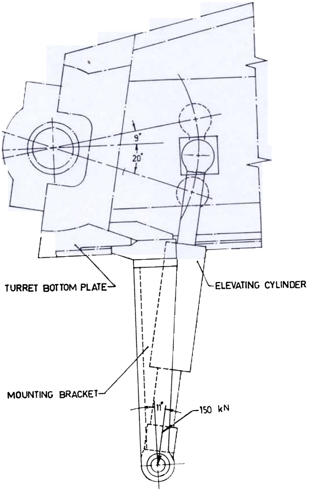
Figure 7. Elevating cylinder mounting.
