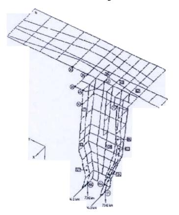
Figure 8. Graphic generated view of elevating cylinder mounting bracket.
