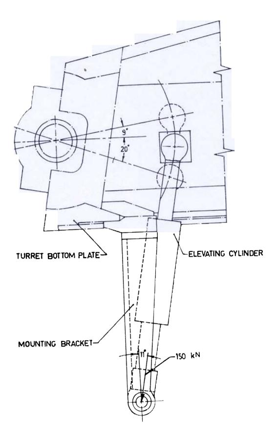
applied as shown in Fig. 8. The deflections obtained at some selected nodes are given in Table 5 and the stresses at some selected elements in Table 6. The node numbers selected are indicated inside the circle and element numbers inside square in Fig. 8. The maximum x-translation at the node 166 is 3.4 mm and maximum stress on the element 103 is 276.4 N/mm<sup>2</sup>. By properly reinforcing the turret bottom plate and bracket, the stresses and deflection can be brought down to allowable range.
