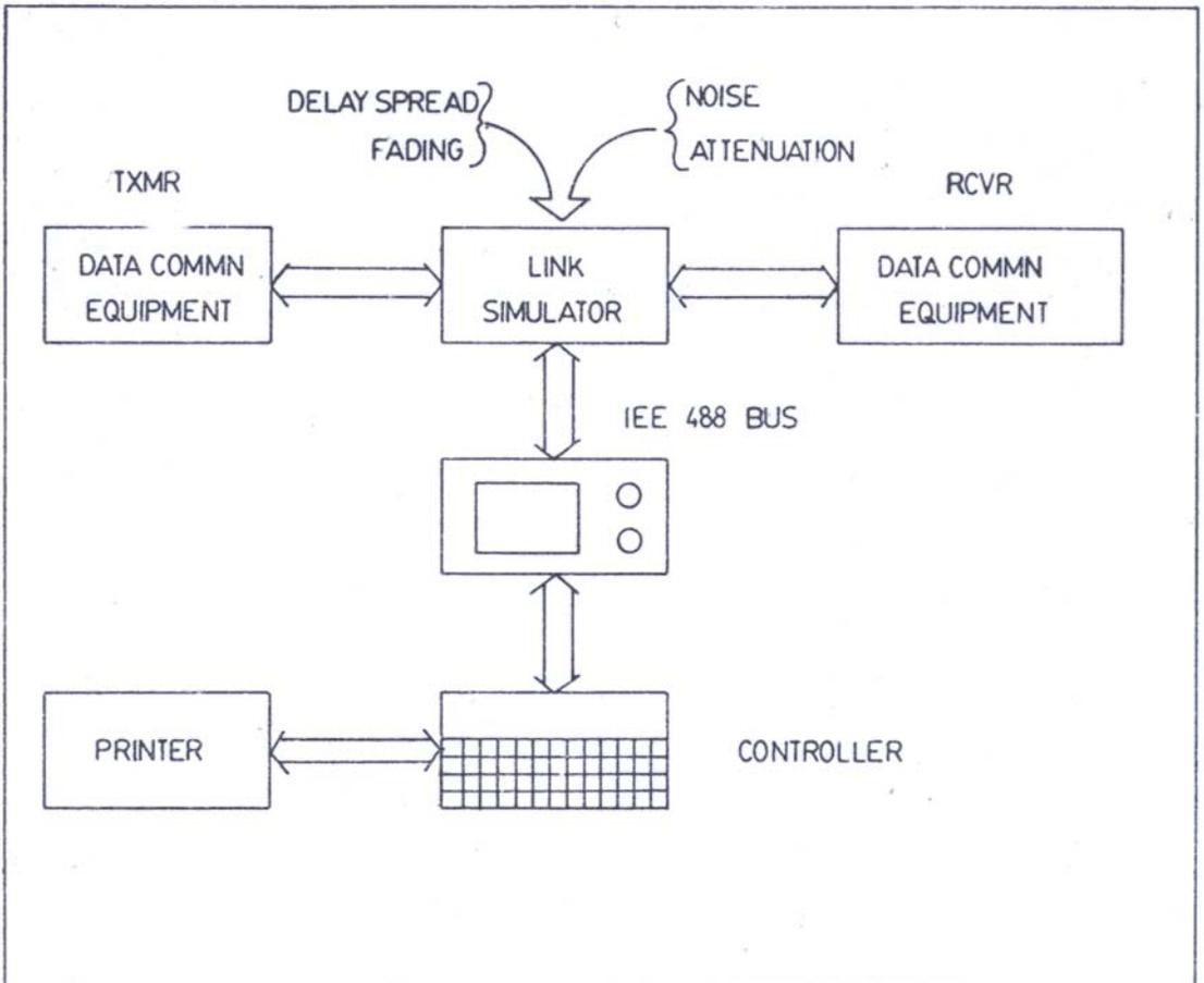
Figure 4. Data communication equipment evaluation.
