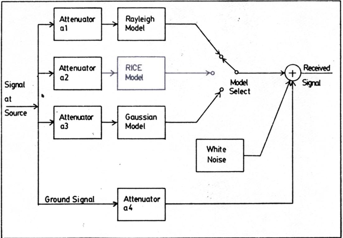
Figure 3. Integrated model of the simulator (single channel).
