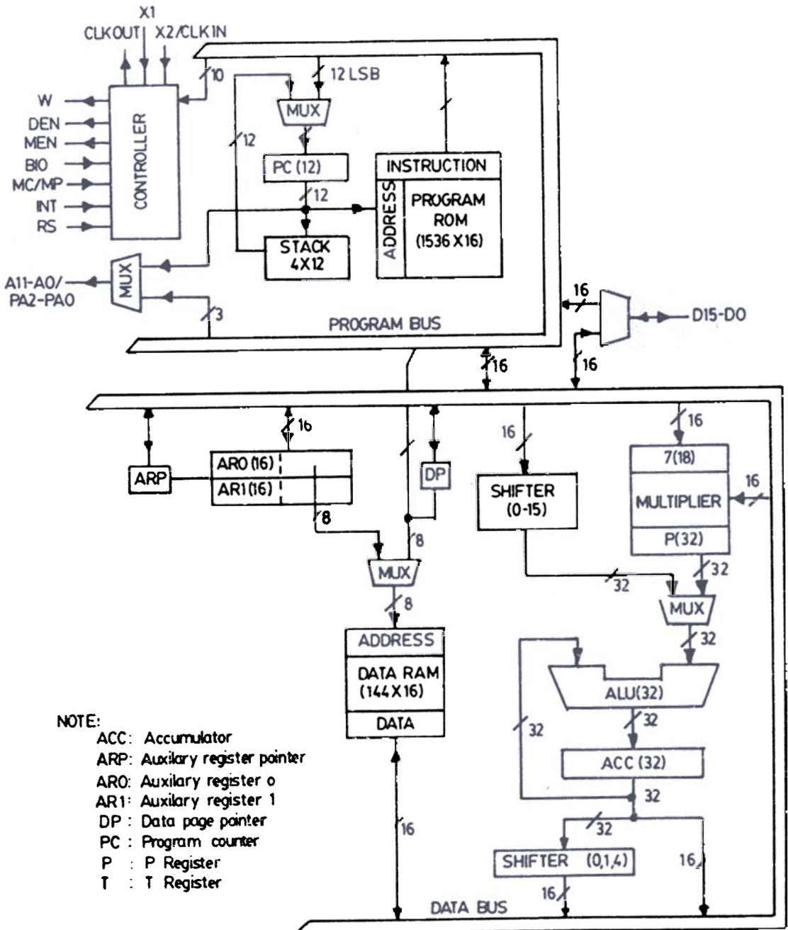
Figure 1. TMS32010 digital signal processor.
