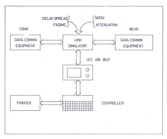
Figure 4. Data communication equipment evaluation.
