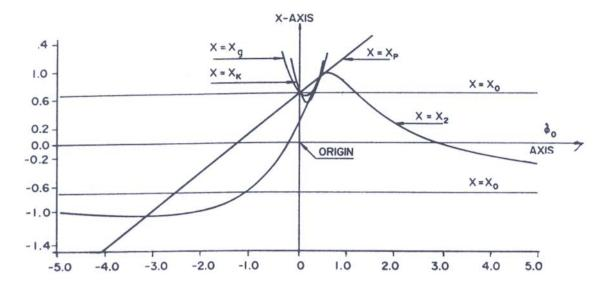
Figure 11. Classification of motion (Lagrangian gravity gyro) ( $\Omega = 1.0$ ;  $X_{\theta} = 0.68$ ;  $\delta_{\theta} = 47^{\circ}$ ; a = 0.42; q = 0;  $\beta = 0.0$  and s = 1.20).
