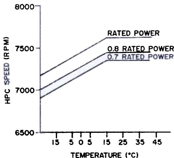
Figure 3. Relationship of speed of HPC and outside air temperature (for recording service life).
