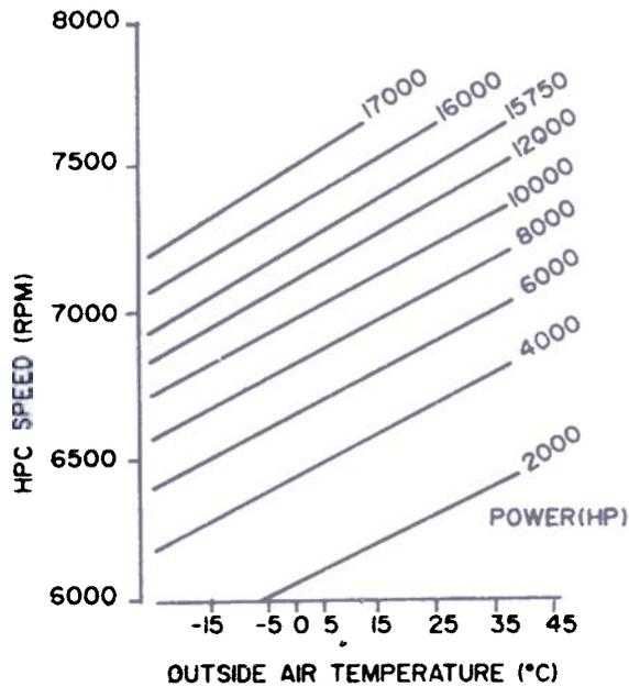
Figure 7. Relationship of speed of HP compressor and outside air temperature (for determination of power).
