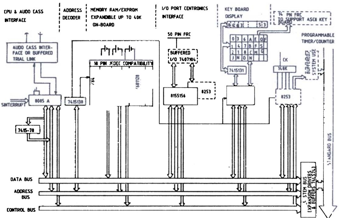
Figure 2. Functional block diagram of a monitoring system.
