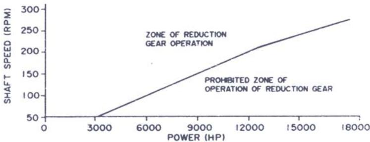
Figure 8. Chart for determination of reduction gear mode of operation.
