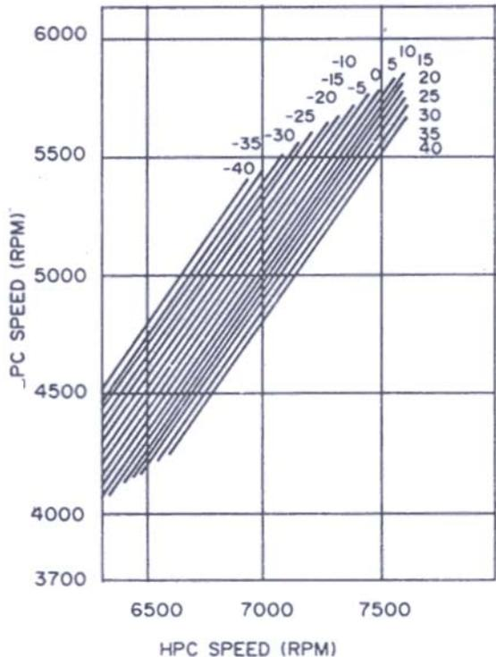
Figure 6. Relationship of speed of LPC and speed of HPC at different temperatures of outside air
