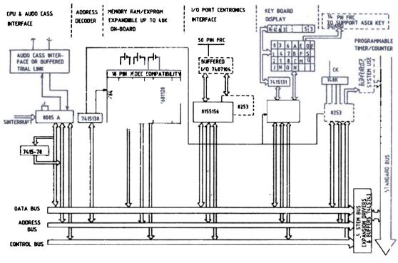
Figure 2. Functional block diagram of a monitoring system.
