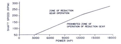
Figure 8. Chart for determination of reduction gear mode of operation.
