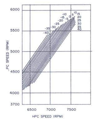
Figure 6. Relationship of speed of LPC and speed of HPC at different temperatures of outside air
