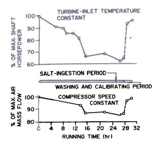
Figure 5. Performance degradation caused by salt ingestion
