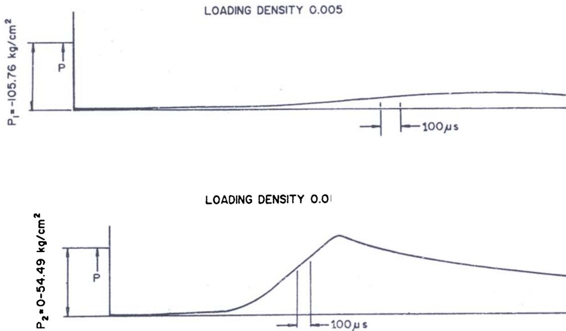
Figure 3. Pressure-time output obtained during DDT experiments at loading density 0.005 and 0.01.
