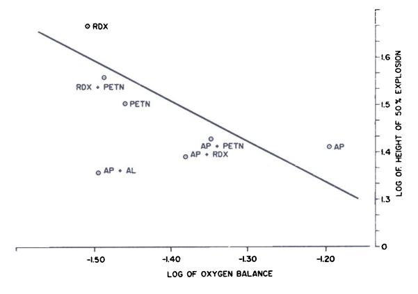
Figure 1. Relationship between impact sensitivity and oxygen balance.
