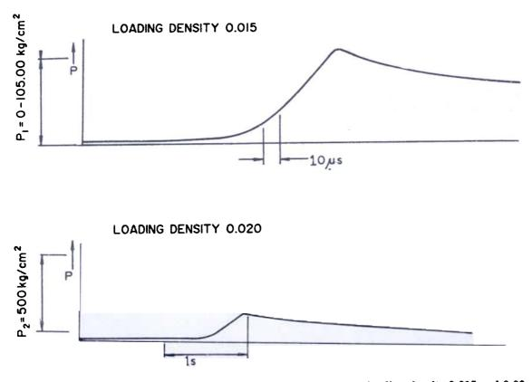
Figure 4. Pressure-time output obtained during DDT experiments at loading density 0.015 and 0.02.
