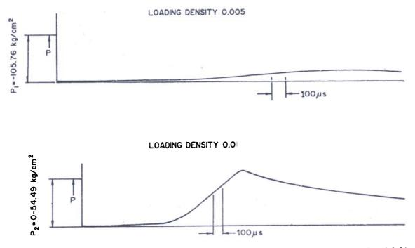
Figure 3. Pressure-time output obtained during DDT experiments at loading density 0.005 and 0.01.
