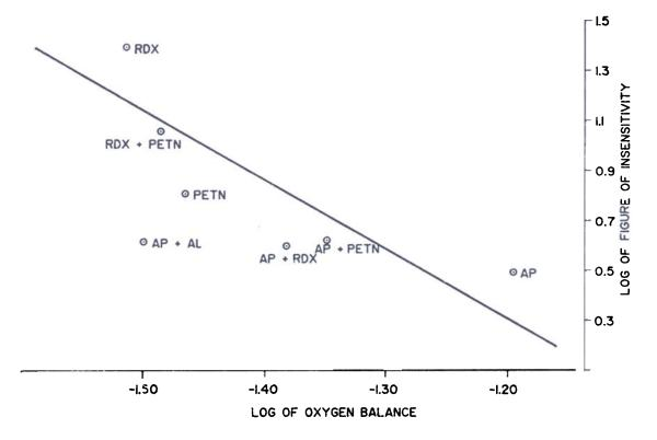
Figure 2. Relationship between friction sensitivity and oxygen balance.
