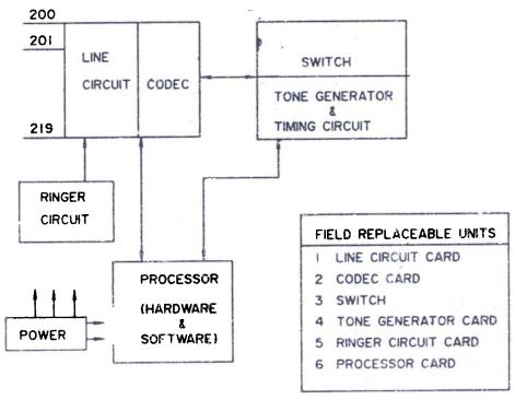
Figure 1 Structural model of the exchange.
