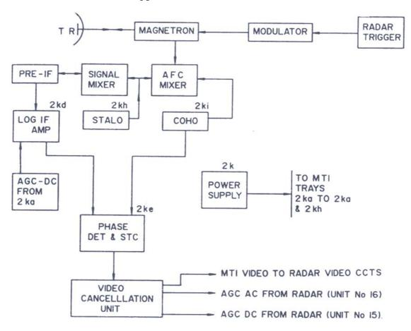
Figure 4. Block diagram of the unit integrated with radar.
