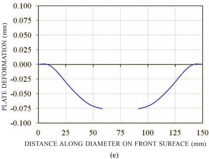
Figure 5. Deformation in target plate in Case-2 analysis for  $V = 830 \text{ m/s}$  at  $t = 1000 \mu\text{s}$ . (a) Deformed armour plate in Case-2 analysis and test<sup>13</sup>, (b) Lateral deformation at centre, and (c) Lateral deformation away from centre.
