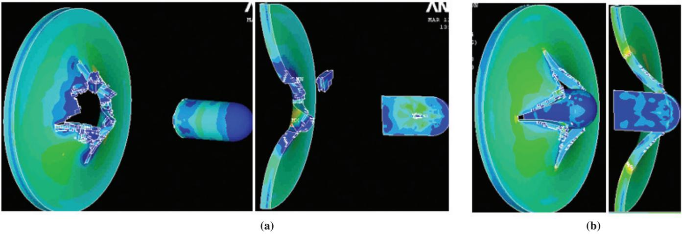
Figure 3. Deformed bullet and target plate at  $t = 50 \mu s$ : (a)  $V = 1000 \text{ m/s}$  and (b)  $V = 500 \text{ m/s}$ .
