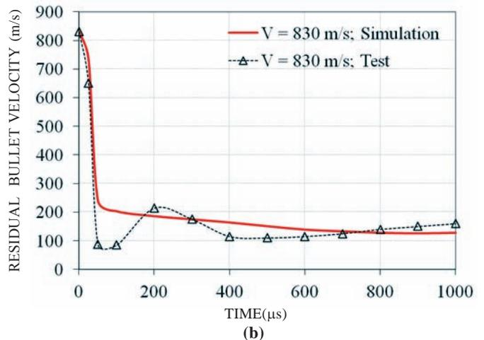
Figure 6. Displacement and residual velocity of AP shot in Case-2 analysis : (a) Displacement and (b) Residual velocity.
