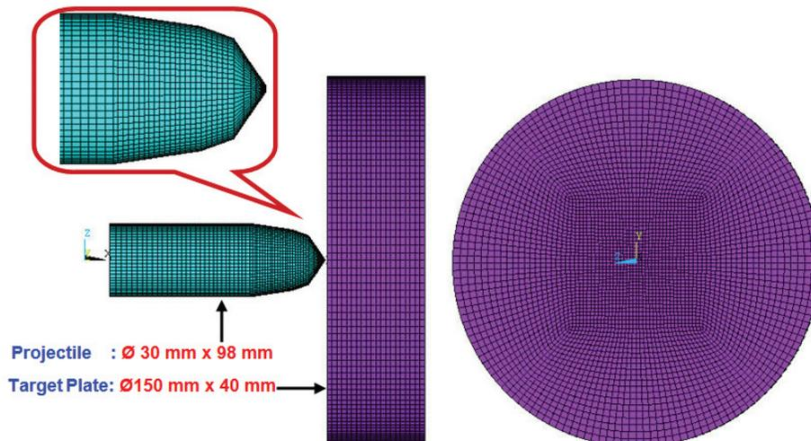
Figure 2. FE model of the AP shot and armour steel target plate for Case-2 analysis.
