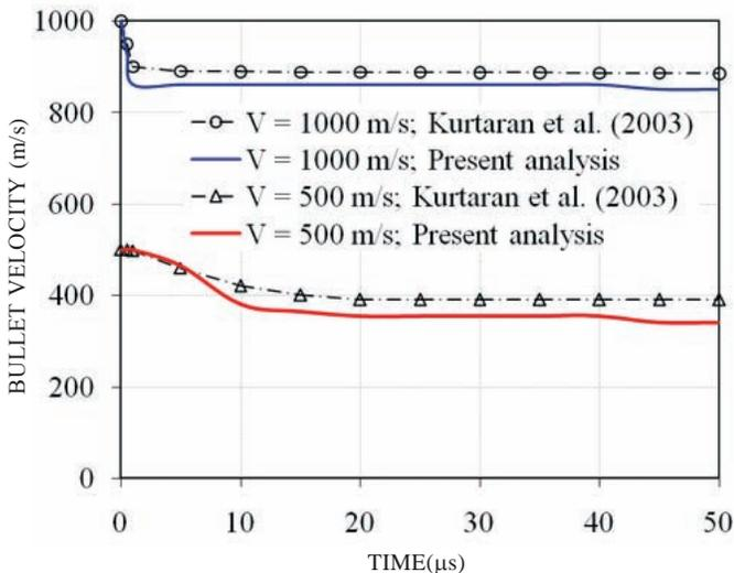
Figure 4. Change in bullet velocity during penetration in Case-1 analysis.
