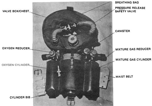
Figure 1. Underwater Breathing Apparatus.
