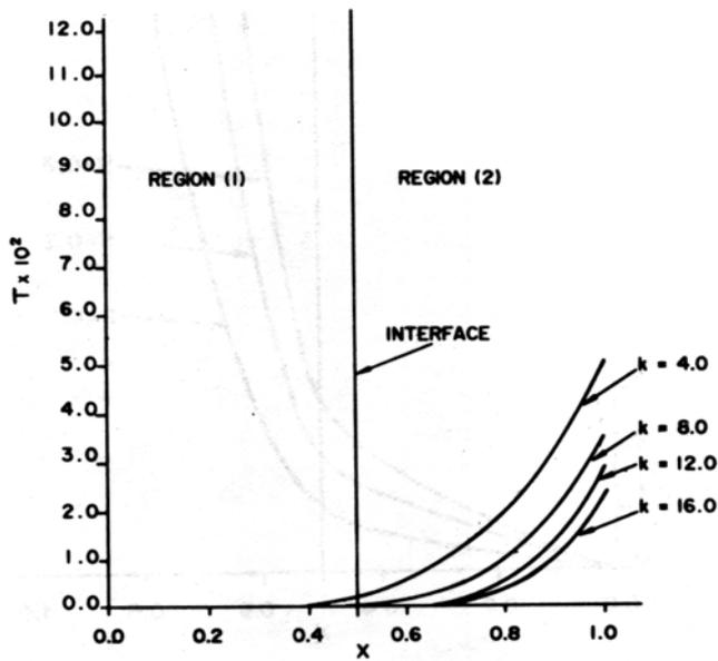
Figure 4. Temperature distribution for various diffusivity ratios at  $s = 0.1, k = 4.0$  and  $\tau = 0.8251$ .
