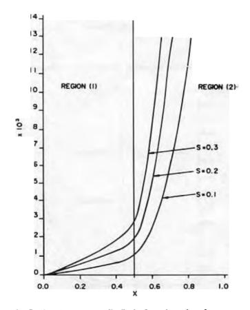
Figure 2. Steady state temperature distribution for various values of source parameter s at K = 4.0 and k = 7.2.
