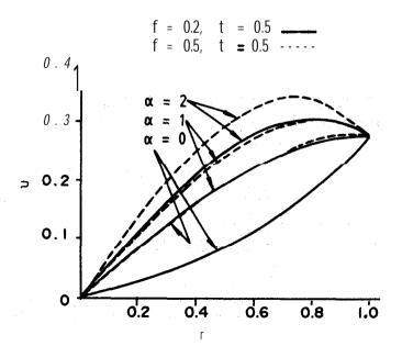
Figure 1. Velocity profile of liquid particles at t = 5 when  $\tau = 0.5$
