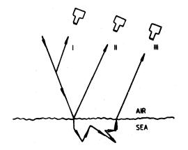
Figure 5. The three sources from which a sensor viewing the sea may receive radiation, viz. the atmospheric back-scattered radiation (I), the surface reflected radiation (II) and the radiation emerging from within the sea (III).
