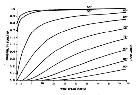
Figure 4. Probability functions of receiving plane polarised light from a wind-roughened sea (wind speeds from 0 to 60 knots) for different look angles varying from 50 to 90 degrees.
