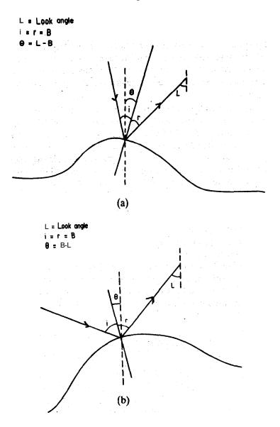
Figure 2 Two possible viewing geometries of receiving a reflected beam from a non-flat sea surface (the diagram is only symbolic and not drawn to scale).
