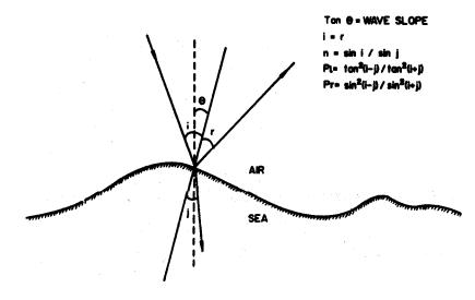
Figure 1. Interaction of an individual ray with the air-sea interface. *Pi* is the parallel component and *Pr* is the perpendicular component of polarisation of reflected beam.
