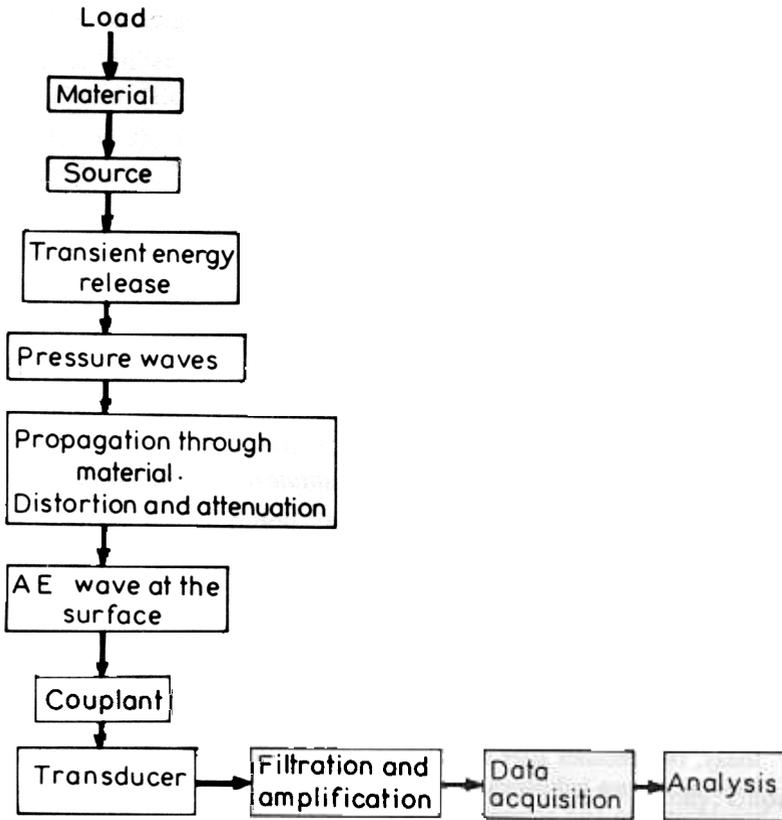
Figure 1. Morphology of AE signals.
