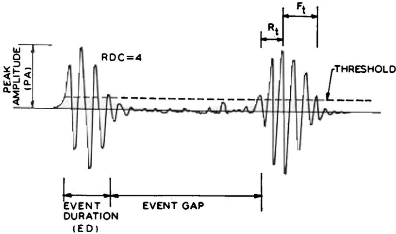
Figure 4. Some AE signal parameters.
